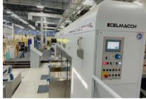
the new Chroma Print offers high performance, both in terms of quality and operation. Printing precision is ensured by direct motor technology thanks to an independent motor on each shaft.
