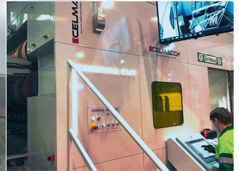
Celmacch HBL rotary die-cutter, fully driven by direct motors. We are very proud to be a trusted supplier to Letro.”
